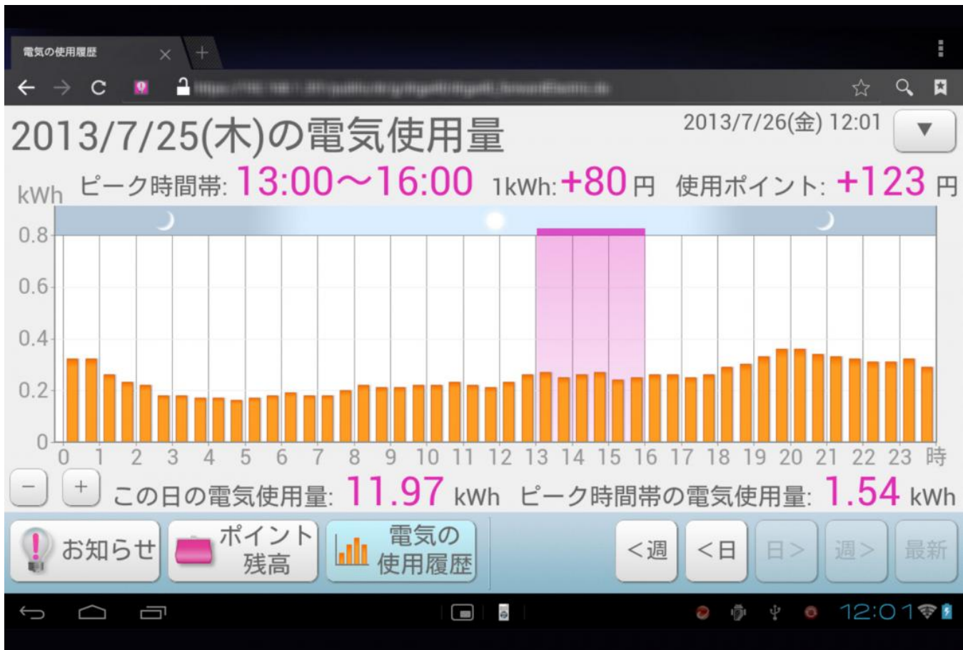
Example of electricity usage information provided by an in-home display. Photo: Fig A.1, Ito et al.
